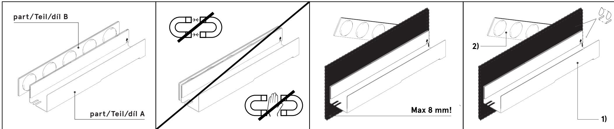
The shelf has two parts equipped with magnets.
